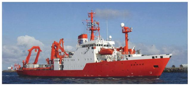
RV SONNE is the oldest but very reliable research vessels of the German fleet usually operating in the Pacific Ocean. With a length of about 98m and a beam of 14 m she has more than 200 m<sup>2</sup> in laboratory space and can host 25 scientists on cruises up to 50 days. For more technical information see: http://www.rf-bremen.de/englisch/sonne.html
