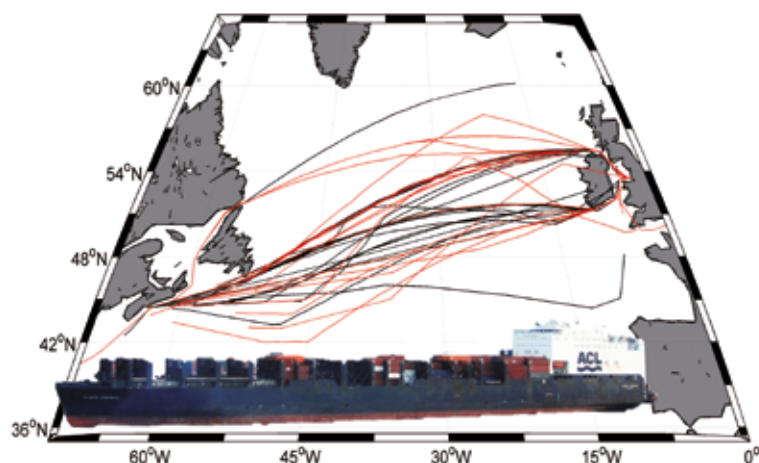
Cruise tracks of M/V Atlantic Companion . While underway it measures carbon dioxide (black and red) and carbon isotopes (red).
