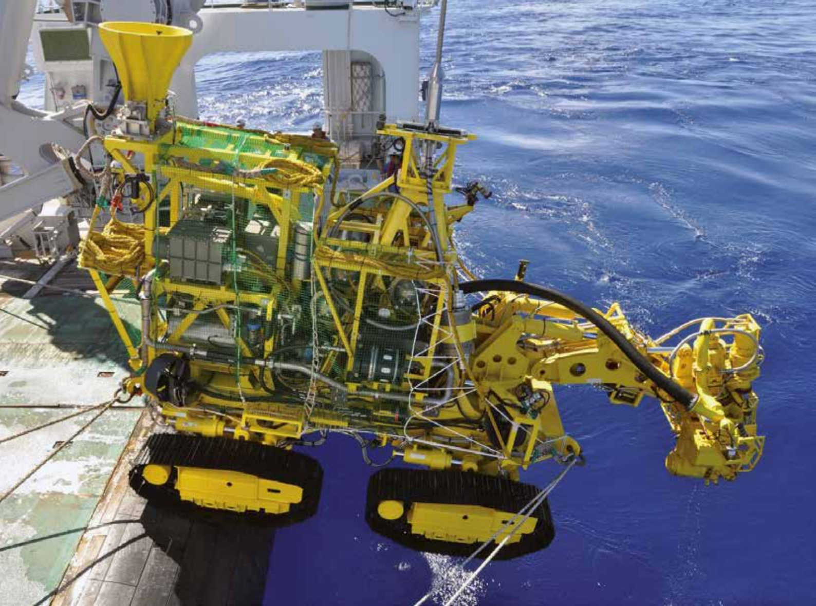
Ore-collecting test machine launched from the deck of a Japanese vessel Copyright: Ministry of Economy, Trade and Industry of Japan.
