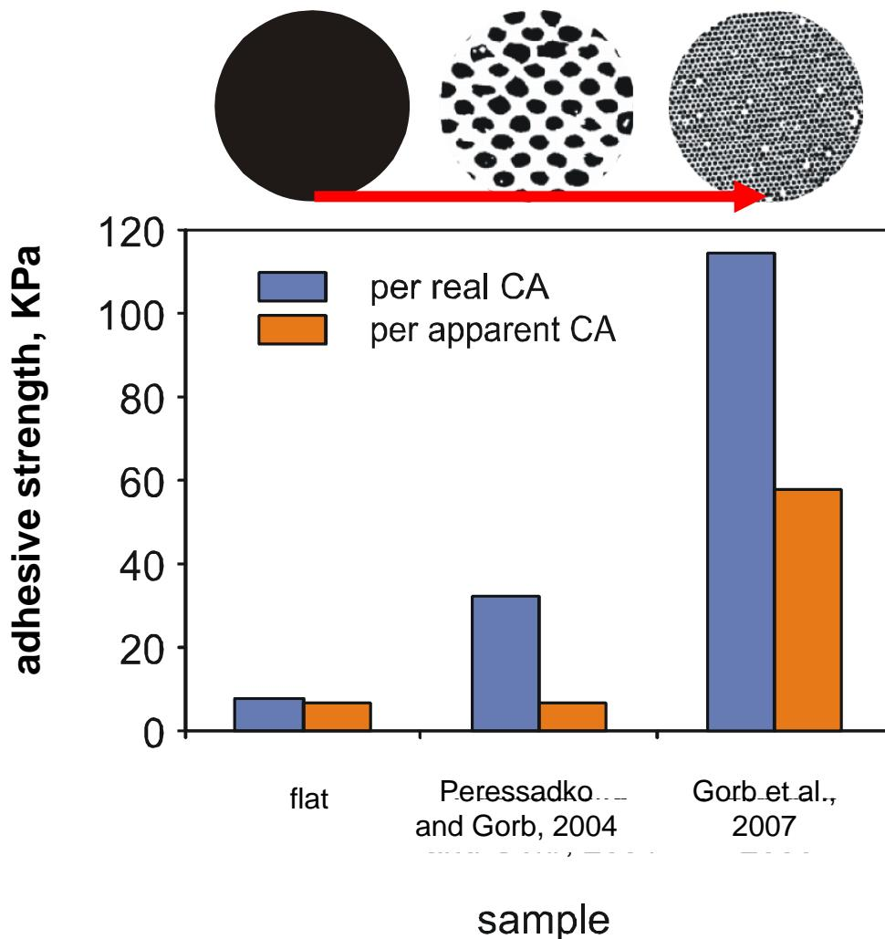
Enhanced adhesion of mushroom-shaped microstructure relies on combination of **van der Waals forces** and **crack-trapping mechanism** (e.g. Hui et al. 2004, *J. R. Soc. Interface*; Carbone et al. 2011, *Soft Matter*)
