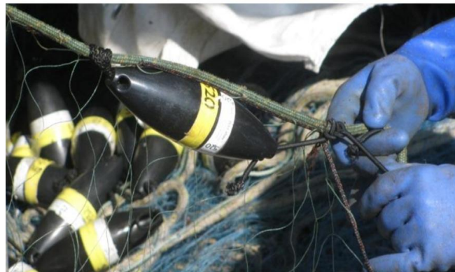
Fig. 4: “PAL” v.1 on the floatline of a gillnet
